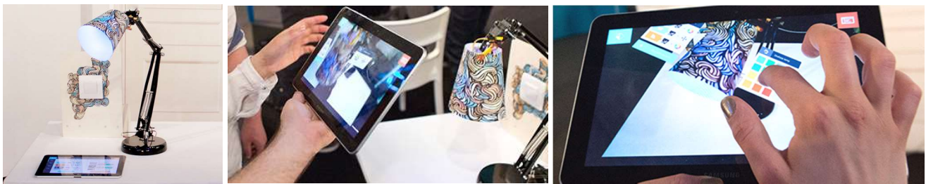
Figure 1. ArLive allow users to create predefined behavior. (Left) ArLive prototype composed of a desk lamp and a light switch. (Middle) People interacting with the prototype. (Right) Close-up of the see-through augmented reality interface.
