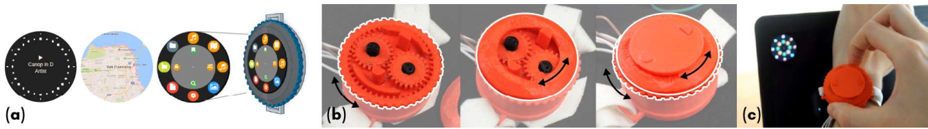
Figure 5: (a) The three implemented applications and the envisioned device. (b) Our proof-of-concept, a watch using two stacked bezels. The bottom bezel is toothed, the top bezel is slanted. (c) For demos, we used a deported screen when visual feedback was necessary
